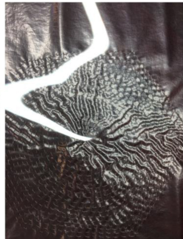
Experiment: embroidered speaker on technical textile
