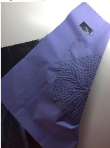
Experiment: embroidered soft speaker on technical textile
