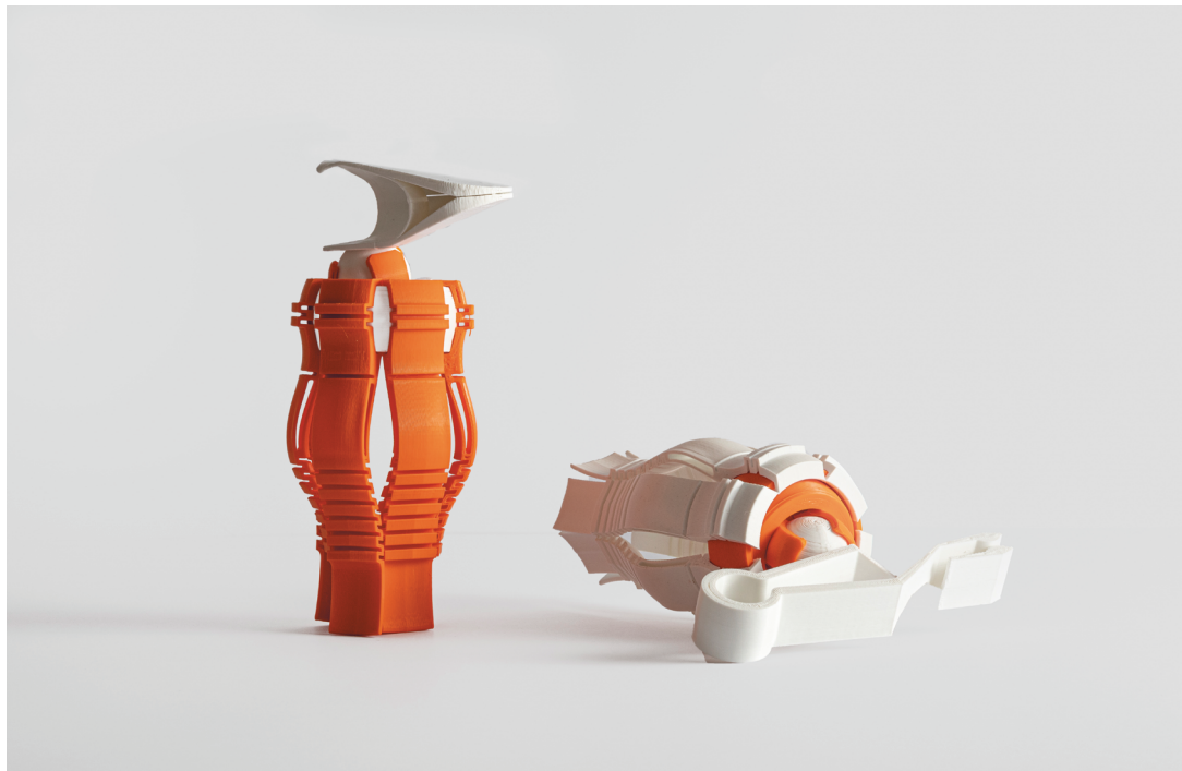
Figure 44: 3D printed modular grasp central pieces with attachments. Photo by Marcell Kazsik.
