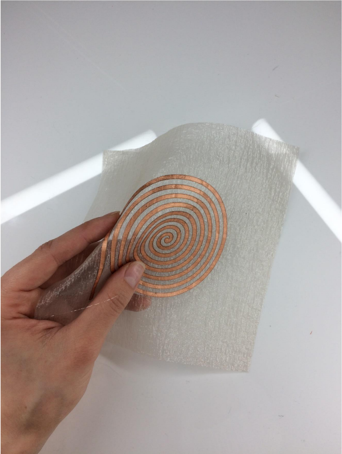
Figure 14: Laser cut copper coil on transparent textile
