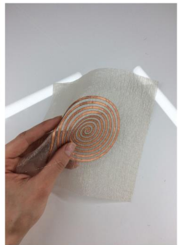
Laser cut coil on transparent textile
