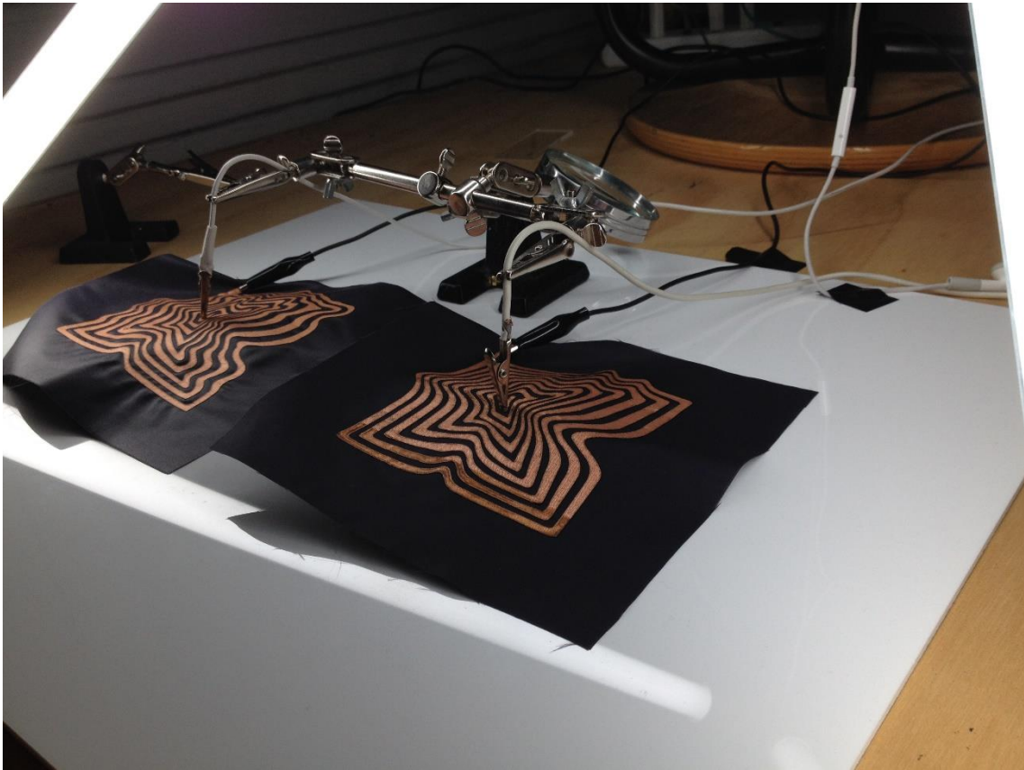
Figure 18: Stereo soft speaker testing at WeMake makerspace, Milan
