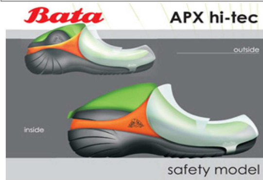
BATA SAFETY SHOE DESIGN CONCEPT, LOW-CUT STEP-IN DESIGN
