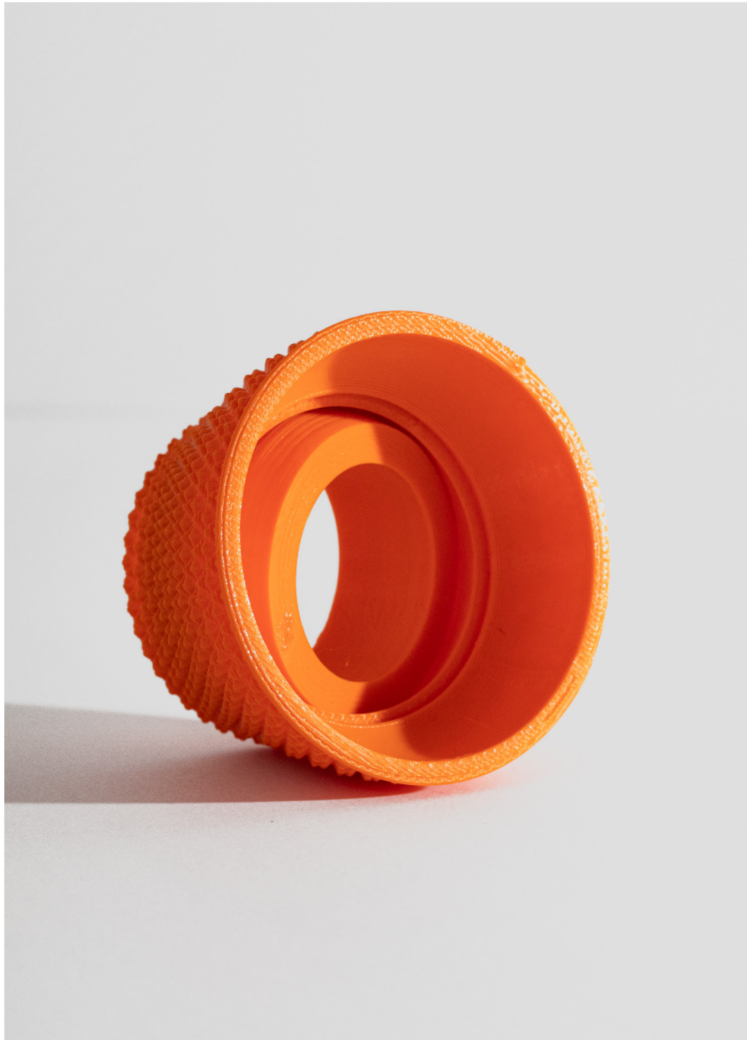
Figure 30: 3D printed bearing gear with the tangible exterior. Photo by Marcell Kazsik.
